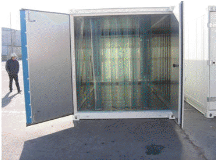
Plastic Curtain in door end
