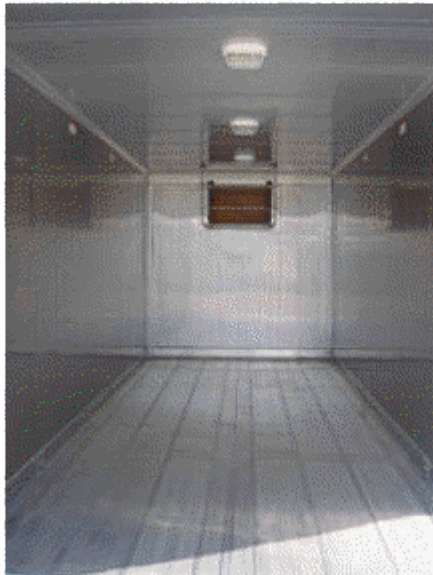
Aluminium Floor w/Pallet guides
